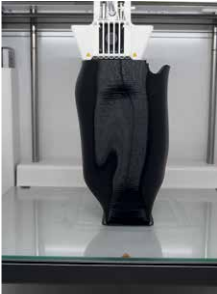
Figure 2. 3D Print of the prosthetic socket with the Ultimaker S5.
