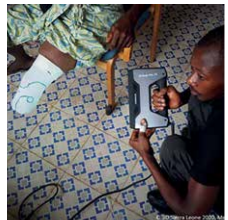
Figure 1. Scanning of the stump with the EinScan Pro Plus.
